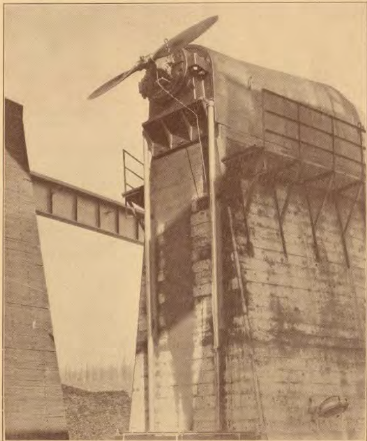
Propeller test rig with propeller mounted and ready for testing
